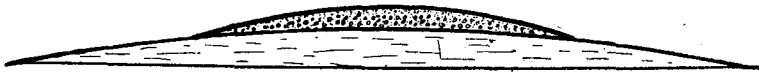
Diagrammatic cross section of road that has been rolled during its construction, leaving a broad, even surface for traffic.
