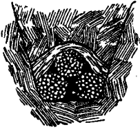
Fig. 10. Subdrain made of bundles of brush for conveying spring water under or alongside roads.
