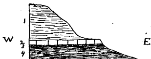
Fig. 8. Profile showing the occurrence of the Rockford goniatite limestone a quarter of a mile west of the center of the east line of Lot 62 of the Illinois Grant. (1) 20 feet of greenish argillaceous shale, typical of the base of the Knobstone group. (2) 18 inches goniatite limestone. (3) 6 inches of soft shale, resembling that overlying the limestone. (4) New Albany black shale.
