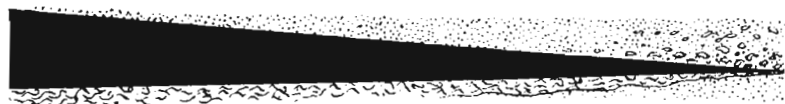
Fig. 822. Figure showing thinning out of Coal VII in Cotterill mine (from sketch by Mr. Kindle).
