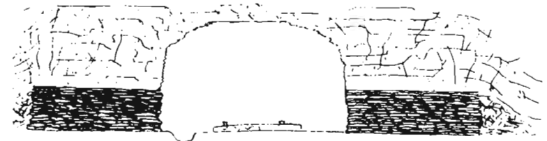
Fig. 959. Same, after gob has settled under weight of roof, and sufficient of the roof has been taken down to give the necessary height in the entry for hauling.
