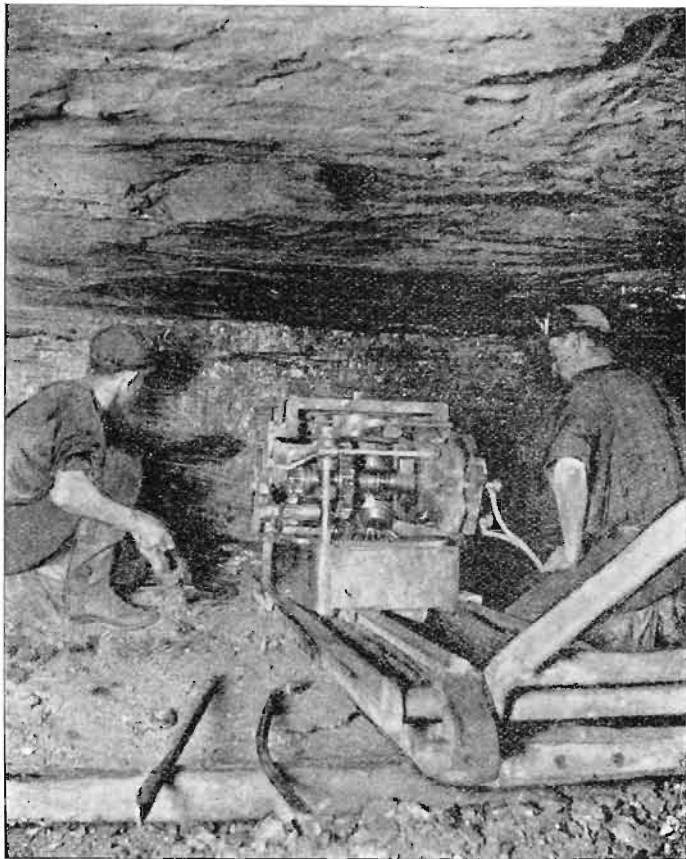
Fig. 970. Electric chain machine at work in Mecca mine. From flashlight photo by Mr. W. Paul Zimmerman.
